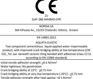
Tensile adhesion strength after heat ageing:  $\geq 0.5 \text{ N/mm}^2$ Tensile adhesion strength after water contact:  $\geq 0.5 \text{ N/mm}^2$ Tensile adhesion strength after contact with lime water:  $\geq 0.5 \text{ N/mm}^2$ Tensile adhesion strength after freeze-thaw cycles:  $\geq 0.5 \text{ N/mm}^2$ Dangerous substances: See product's SDS
