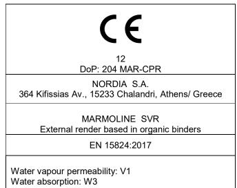
Water absorption: W3 Adhesion:  $\geq 0.80$  MPa Thermal conductivity :  $\lambda_{10}$ ,dry = 0,83 W/mK (tab. mean value; P= 50%) Reaction to fire: A2-s2, d0
