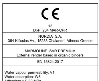
Adhesion:  $\geq$  0.80 MPa Thermal conductivity: 1 & 1.5 mm:  $\lambda_{10}$ ,dry =0.83 W/mK 2 & 3 mm:  $\lambda_{10}$ ,dry =1.17 W/mK (tab. mean value; P= 50%) Reaction to fire: A2-s2, d0
