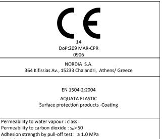
$\begin{array}{ll} \mbox{Crack bridging properties} \\ \mbox{(Method A - Static)} & : A4 ( -10^{\circ} C ) \\ \mbox{(Method B - Dynamic)} & : B2 ( -10^{\circ} C ) \\ \mbox{Capillary absorption and permeability to water : w< 0.1 kg/m^{2}h^{0.5} \\ \mbox{Dangerous substances: } comply with §5.3 \\ \mbox{Reaction to fire: B2-s1,d0} \end{array}$
